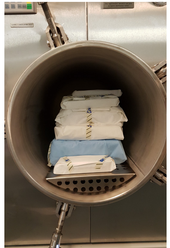
The autoclave prototype being packed during field testing in Haiti.
