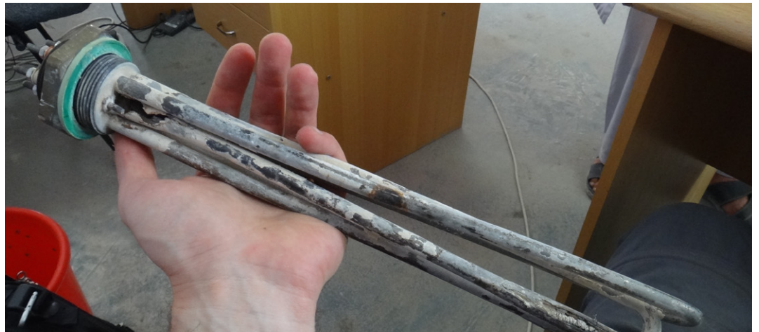
Universities were involved to analyze broken heater elements from autoclaves used in the field.
