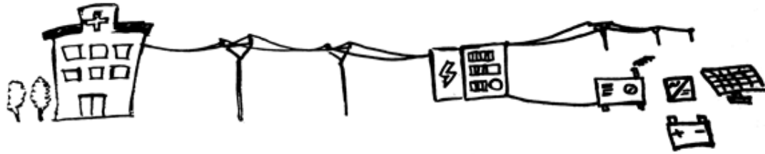
FIGURE 2. LOCAL ELECTRICITY SYSTEM OF A PROJECT, WHERE THE NEEDS FOR SERVICE NECESSITATE A POWER DISTRIBUTION SYSTEM FED BY AN ON-SITE GENERATOR OR BY CONNECTION TO AN EXTERNAL GRID.
